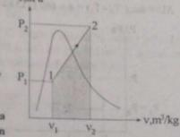
13. Oxygen (4 kg) is contained in a piston cylinder device shown in figure below initially at a pressure of 1000 kPa and a temperature of 77° C. There is a heat transfer to the system until the piston reaches the upper stops, at which time volume inside the cylinder is 0.6 m3. The oxygen is further heated until the pressure reaches to 2000 kPa. Sketch the process on P-V and T-V diagrams and determine the total work and heat transfer in the process. [Take R = 260 J/kgK and c, = 660 J/kgK
