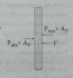
For the piston cylinder device shown 14. in figure below, determine the force necessary to produce an absolute pressure of 500 kPa within the device. [Take Patm = 100 kPa]
