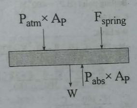
Referring to the free body diagram of the piston we can write equation for the pressure inside the cylinder as
