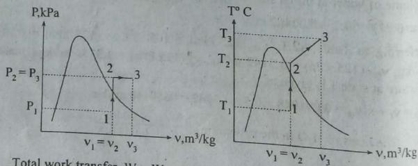
Total work transfer,  $W = W_{12} + W_{23} = 0 + P_2 (V_3 - V_2)$ =  $mP_2(v_3 - v_2) = 0.006714 \times 600 (0.8246 - 0.688148) = 0.5497 \text{ kJ}$  23. A piston cylinder device shown in figure below contains 2 kg of water initially at a pressure of 500 kPa with a quality of 20 %. The water is heated until it becomes a saturated vapor. The volume of the system when the piston is at the upper stops is 0.4 m3. Sketch the process on P-v and T-v diagrams and determine:
