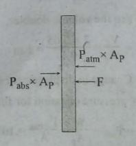
A piston cylinder device loaded with a linear spring with a spring constant of k = 100kN/m contains a gas initially at a pressure of 100 kPa and a volume of 0.05 m<sup>3</sup>, as shown in figure below. The cross sectional area of the piston is 0.01 m2. Initially spring touches the piston but exerts no force on it. Heat is supplied to the system until its volume doubles, determine the final pressure. (IOE 2068 Bhadra)
