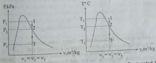
19. A 0.05 m<sup>3</sup> rigid vessel initially contains a mixture of saturated liquid and saturated vapor at 100 kPa. The water is now heated until it reaches the critical state. Determine the mass and volume of the saturated liquid water at initial state.
