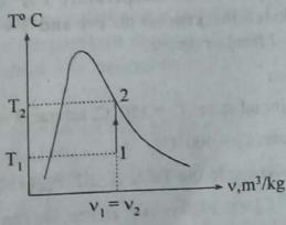
14. A rigid vessel with volume of 0.4 m<sup>3</sup> contains 2 kg of water in the form of saturated liquid and saturated vapor mixture. Heat is supplied t the system from an external source. Determine the temperature at which the water in the vessel is completely vaporized.
