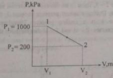
Final state:  $P_2 = 200 \text{kPa}, V_2 = 0.2 \text{ m}^3$
