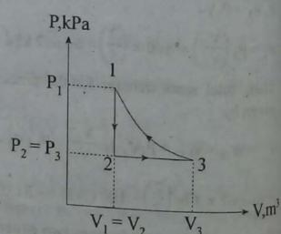
$$W = W_{12} + W_{23} + W_{31} = P_2 (V_3 - V_2) + P_3 V_3 \ln \left( \frac{V_1}{V_3} \right)$$
