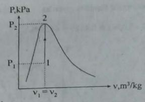
20. A piston cylinder device shown in figure below contains 0.5 kg of water initially at a pressure of 1 MPa and 250° C. Heat is lost by the system until it becomes saturated liquid. Sketch the process on P-v and T-v diagrams and determine the work transfer.
