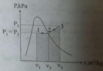
Solution of Fundamentals of Thermodynamics and Heat Transfer | 8 W = W<sub>12</sub> + W<sub>23</sub> = P<sub>1</sub> (V<sub>2</sub> - V<sub>1</sub>) +  $\frac{1}{2}$  (P<sub>2</sub> + P<sub>3</sub>) (V<sub>3</sub> - V<sub>2</sub>) = 100 (0.015 - 0.01) +  $\frac{1}{2}$  (100 + 200) (0.015312 - 0.015) = 0.5468 kJ
