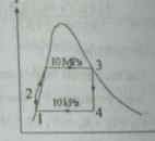
State 1: P<sub>1</sub> = 10kPa, saturated liquid
