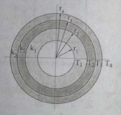
wat transfer per unit length for the composite cylinder is then given by
