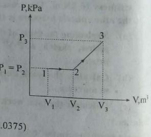
sketch the process on P-V diagram. Both springs have spring constant of 100 kN/m.
