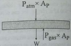
Initial pressure of the system is 100 kPa and pressure required to lift the piston is 149.05 kPa. Hence, during initial stage of heating piston remain stationary although heat is supplied to the system, so process is constant volume heating (Process 1-2). During constant volume heating, pressure of the system increases from 100 kPa to 149.05 kPa. Hence, we can define state 2,
