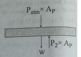
Thus, pressure required to lift the piston (Plift) = 500 kPa
