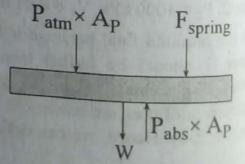
Initially spring touches the piston the piston but exerts no force on it. Substituting initial state ( $F_{spring} = 0$ ) on the pressure equation, we get
