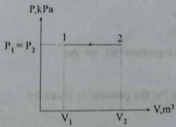
$$W = P_1 (V_2 - V_1) = 150 (0.1 - 0.04) = 9 \text{ kJ}$$
