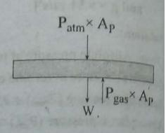
12. A pisotn cylinder has a diameter of 0.2 m. with an outside atmospheric pressure of 100 kPa, determine the piston mass that will create at inside pressure of 500 kPa. [Take  $g = 9.81 \text{ m/s}^2$ ]
