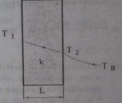
44. A 2 m long steel pipe (k= 50 W/mK) is well insulated on its sides, while its left section is maintained at 100° C and the right section is exposed to ambient air at 20° C. Under steady state conditions, a thermocouple inserted at the middle of the plate gives a temperature of 80° C.
