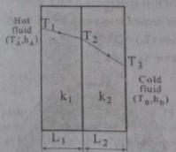
Heat transfer per unit area for a composite plane wall subjected to convection on both sides is given as
