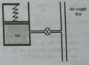
$m^3$ . The valve is opened to let some air in, causing the piston to rise 5 cm. Find the new pressure. [Take  $g = 9.81 \text{ m}^2/\text{s}$ ]
